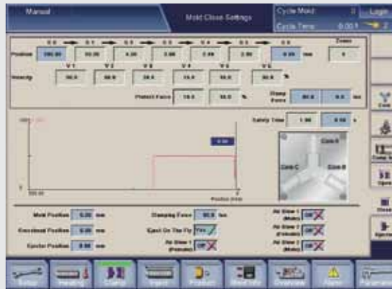
Mold protection function with 2 steps in standard.
